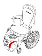
Normally, when getting out of the wheelchair the footrest is tilted up. The footrest is designed that one does not need to tilt it up when one wants to exit the chair. Placesimply your feet's on the outside of the footrest when you want to get up.
