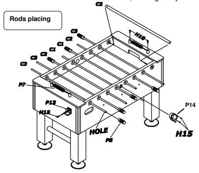
6) Lock Player C8, C9, Goalie rod stop ring C11 on player rods by screw C6 & Nut C7, then inserting two washer C5 on both sides of Rubber bushing C4 as FIGURE 6. Finally, put rod end caps P6 on another side of player rod.
