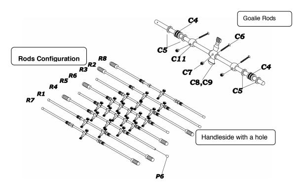
Attention – again please final control that all screws are fixed with a hand screw drive or automatically screw driver with the lowest setting. To place the handles on the rods, please use a simple rubber hammer.
