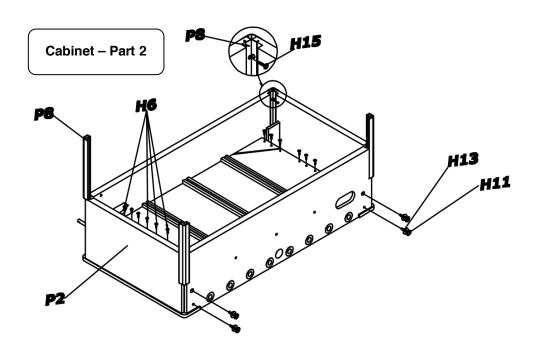
**Attention** – please make sure that in this step now all screws final fixed by hand or within a screw driver or automatically screw driver with the lowest setting.
