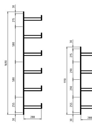
III. 2: Mounting dimensions (drilling holes dimensions)
