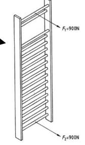
First, fix the mounting brackets to the wall. The mounted wall bars must stand on the floor. See the illustration for drilling measurements on the wall and the sides. The wall bars do not have any pre-drilled holes because on-site conditions such as electrical wiring, pipes and others, could make mounting impossible. The height information for the mounting brackets (wall plugs) is approximate. The horizontal distance between the mounting brackets must be 880 mm.
